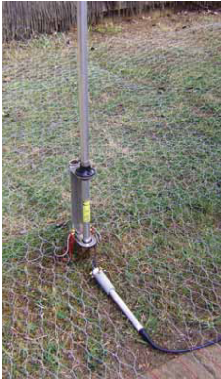
PHOTO 1: ZL1VL's 400 sq ft (37m 2 ) of galvanised chicken wire counterpoise system, which gave a definite all round improvement to the performance of the Hustler 6BTV.
